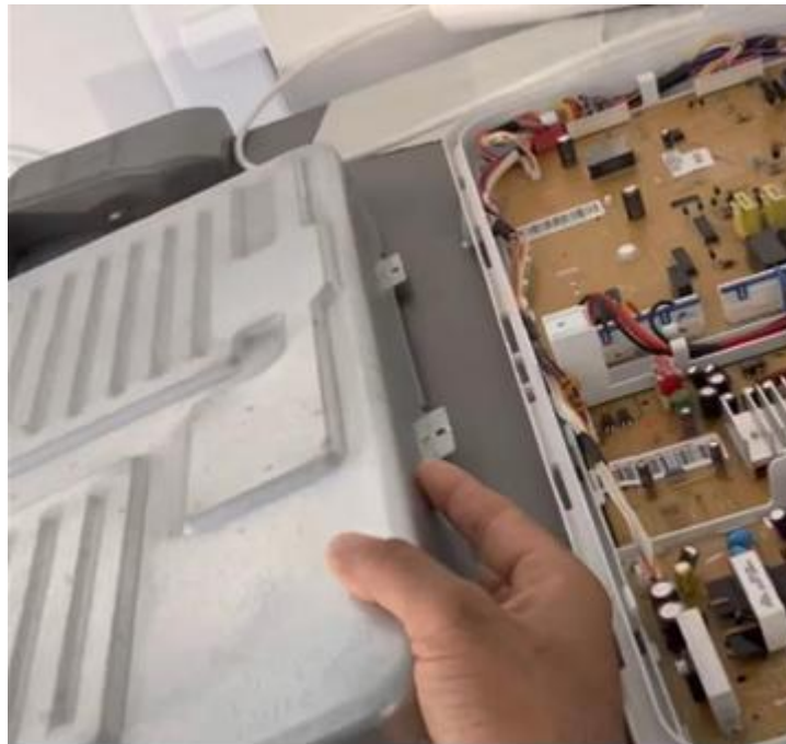
Figure 31: Example of a side-by-side fridge model with electronic boards easily accessible on top of the fridge
